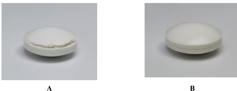
Figure 7. Tablet presenting (A) capping or (B) delamination [65].
