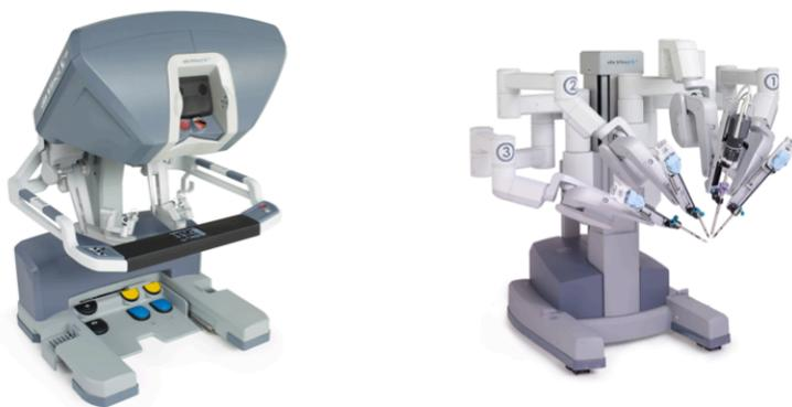
**Abb. 1: Konsole (links) und Patient Cart (rechts) des Da Vinci Si Systems, [www.intuitivesurgical.com/company/media/images/](http://www.intuitivesurgical.com/company/media/images/) (14)**
