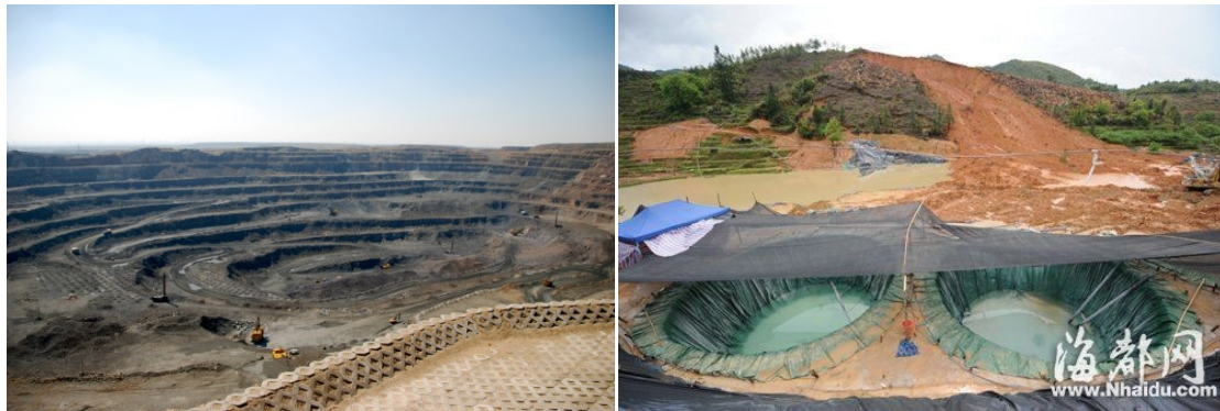
Figure 3–6: The Bayan Obo open-pit mine (left) and sedimentation ponds in Fujian (right) (Sources: Dijk 2011; Tang XZ et al. 2012).
