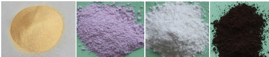
Figure 3–7: Monazite concentrate; neodymium carbonate, cerium chloride, terbium oxide (from left to right). Sources: Guangxi Qinzhou Jinlianda 2013; Jiangsu Guosheng REE 2013.
