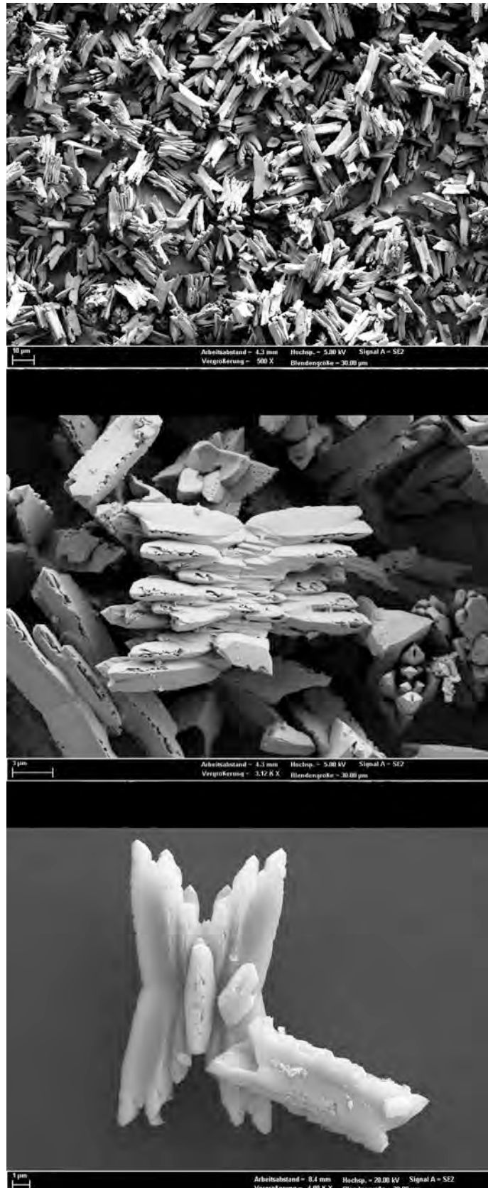
B 1: Barite precipitated from a 5 molal NaCl solution.
