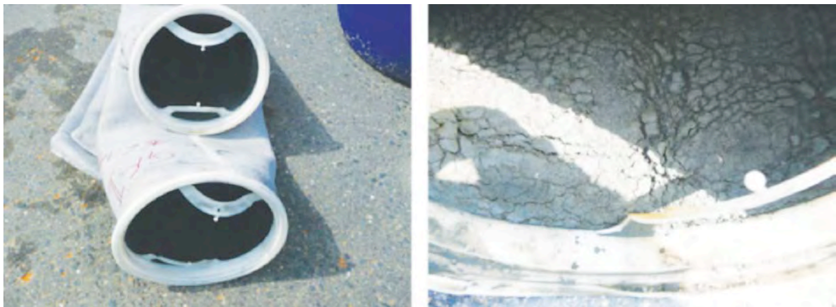
Figure 2.2: Filter bags (left) and close-up of filter residue (right) from the GrSk in-line filtration system. Filters with pore sizes of 10 µm and 2 µm remove suspended solids from the brine before it enters the heat transfer section of the geothermal loop
