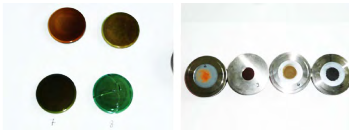
Figure 2.3: Examples of prepared samples for filter residue chemical analysis via XRF (left) and filter residue mineralogy analysis via XRD (right). The high Cl and organic content of the filter residue caused some of the XRF glasses to fracture, as shown in the lower right hand (green) XRF sample
