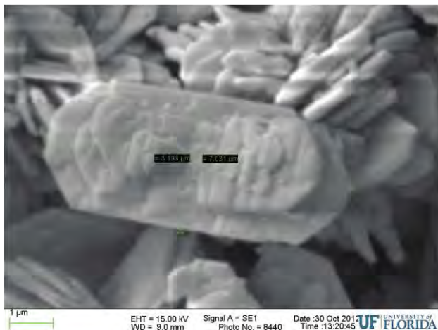
Figure 4.9: Evolution of crystal morphology and estimates of specific reactive surface for strontio-barite crystals precipitating after 0.5, 2 and 4 hours at 150° C.
