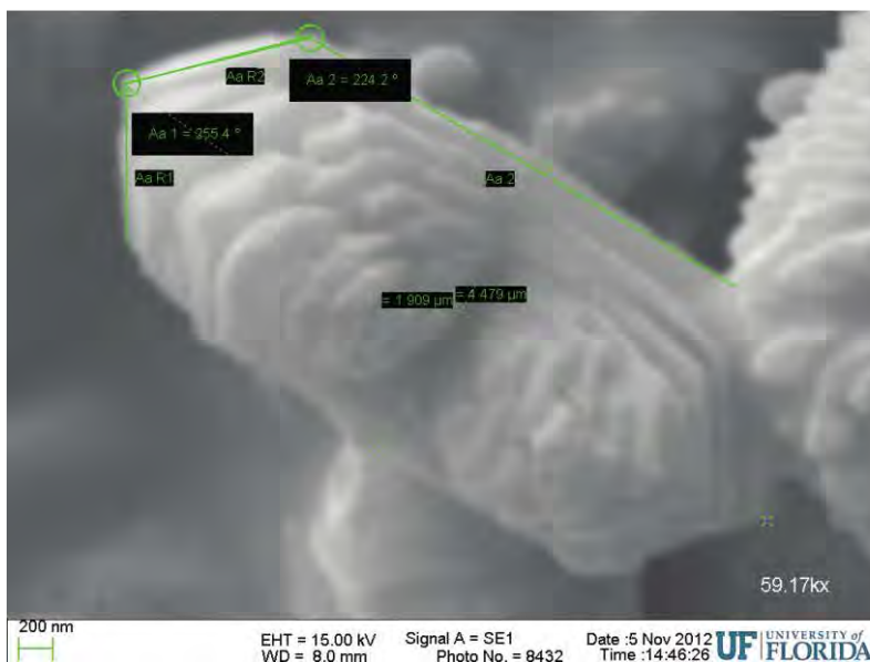
Figure 4.8: Evolution of crystal morphology and estimates of specific reactive surface for strontio-barite crystals precipitating after 0.5, 2 and 4 hours at 75° C.
