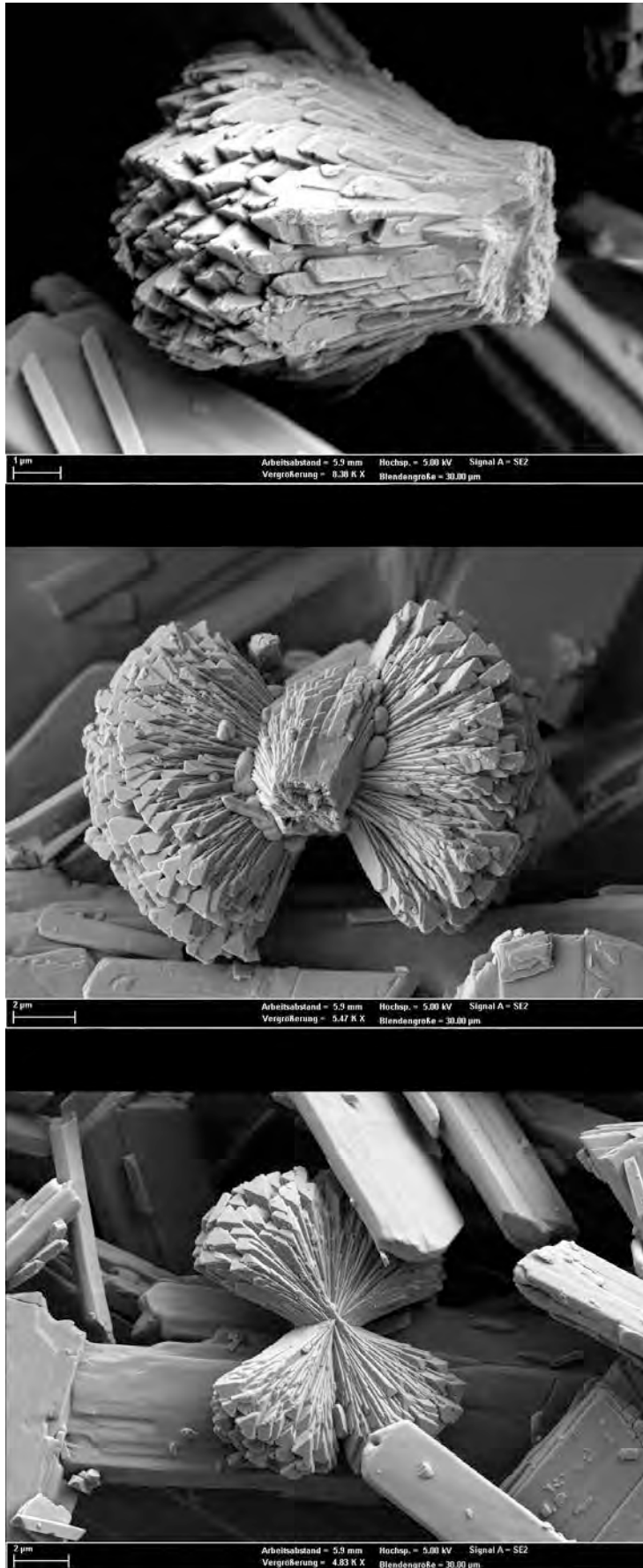
B4 cont: Strontio-barite with anhydrite precipitated from a mixed electrolyte (Na-Ca-Ba-Sr-Cl-SO 4 -H 2 O; 5 molal Cl) solution at GrSk concentrations.
