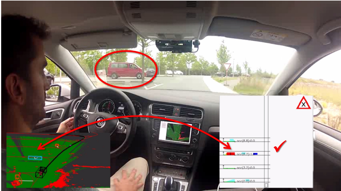
Figure 5.8.: Example of a not successful occurrence due to a function error. The red vehicle (remarked with a red ellipse) was correctly detected and matched to the RG, but due to a function error, the ego vehicle do not react as expected.
