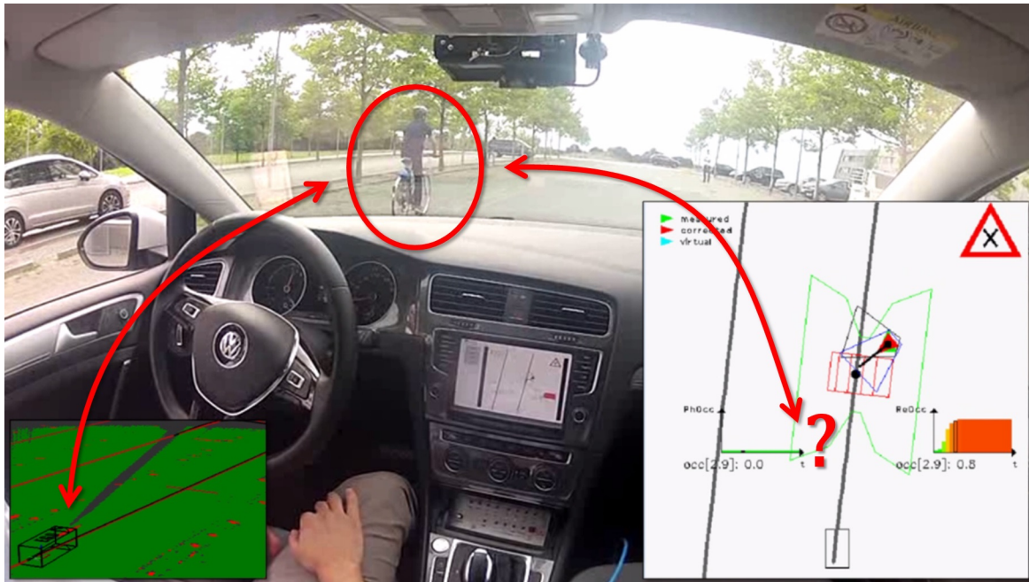
Figure 5.6.: Example of a not successful occurrence due to an object fusion error. A cyclist (remarked with a red ellipse) approaches a crosswalk but is not detected from the sensor fusion. See Fig. A.6 and A.7 for a detailed description of the meaning of the images.
