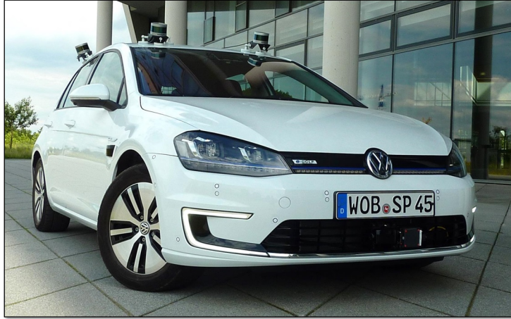
Figure 3.3.: Mounted sensor setup in the demonstrator vehicle (Volkswagen E-Golf 7).
