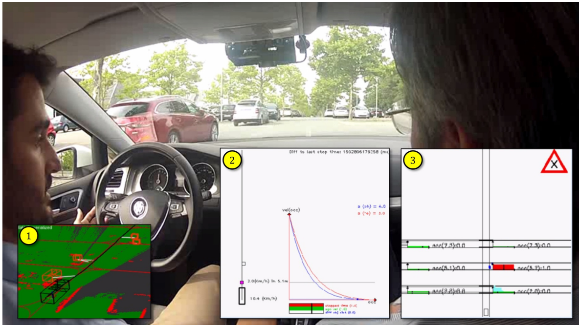
Figure A.5.: Example of a video with 3 developer views, in which the ego vehicle is approaching a right-before-left intersection while an occlusion impedes to observe if a crossing vehicle is coming from the right (occurrence type (o) according to subsection 5.1.2). The displayed developer views are: (1) RG, (2) occlusion handling and (3) vehicles motion prediction.
