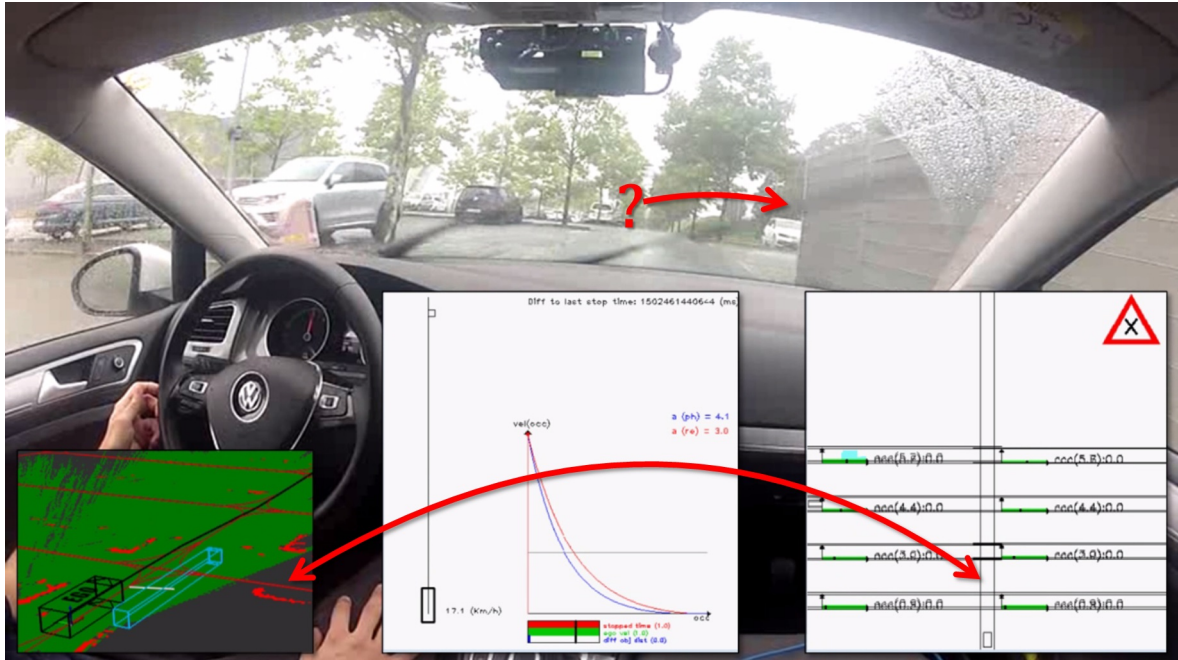
Figure 5.9.: Example of a not successful occurrence due to a wrong parameter value. The ego vehicle approaches a right-before-left intersection but the fence at the right side impedes to perceive if a cross vehicle comes or not (see red arrow and question mark). Due to an erroneously set parameter, the ego vehicle dot not react as expected.
