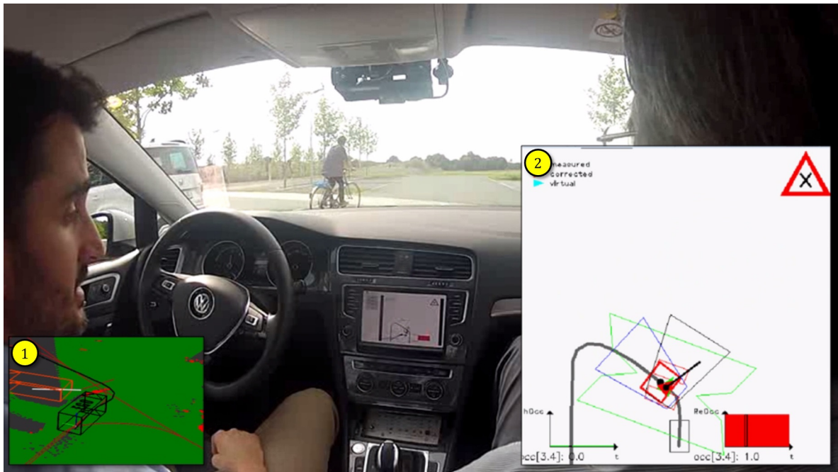
Figure A.4.: Example of a video with 2 developer views, in which a cyclist is crossing a crosswalk in front of the ego vehicle while turning left (occurrence type (e) according to subsection 5.1.2). The displayed developer views are: (1) RG and (2) pedestrians motion prediction.
