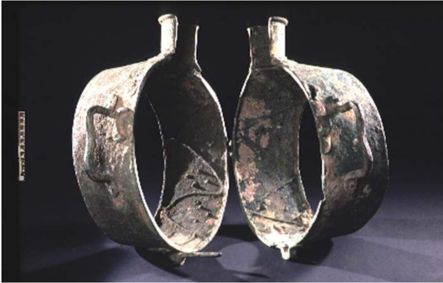
Fig. 3 Bronze sand casting flask from Iran, unknown date. The ingate for pouring in the metal is at the top. Note the relief keying on the inner face. Diameter: 31 cm.
