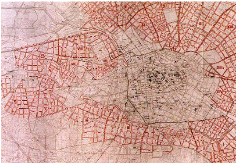
Figure 4. City of Berlin Development Plan by Hobrecht, 1862, featuring sewer network corresponding with planned street network and land lots for development (Aust and Stark 1987).
