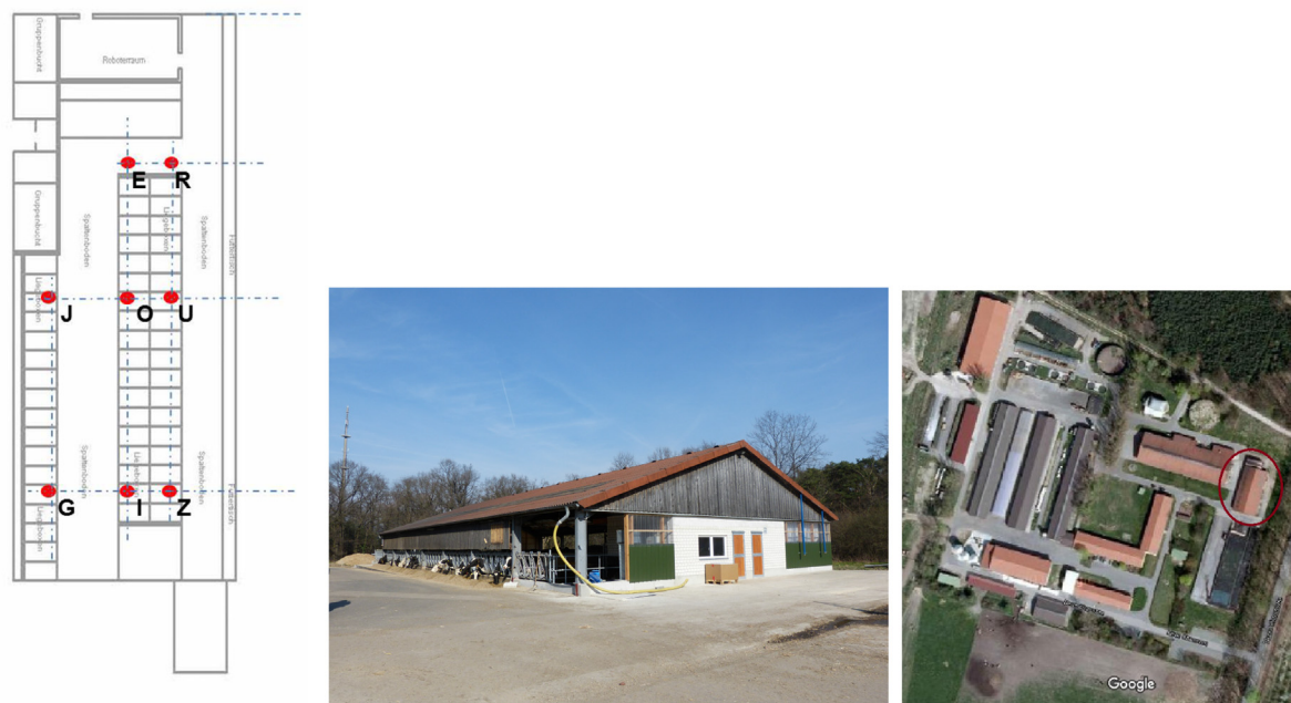
Fig. 2 – Description of the measurement site Gross Kreuzt: Layout of the barn (north front at the bottom of the map) and sensor positions (left), photography of the barn viewed from the main prevailing wind direction (middle, source: ATB) and a map of the farm indicating the position and orientation of the barn (right, source: Google maps).
