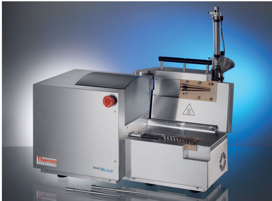
Figure 1.7. Thermo Scientific HAAKE MiniLab II, a Micro Compounder with conical twin-screws (Picture taken from www.rheologysolutions.com )
