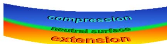
Figure 2.1.1) The upper part of an elastic plate is compressed and the lower part extended. In the middle plane occurs no tension, therefore this plane is called neutral surface.
