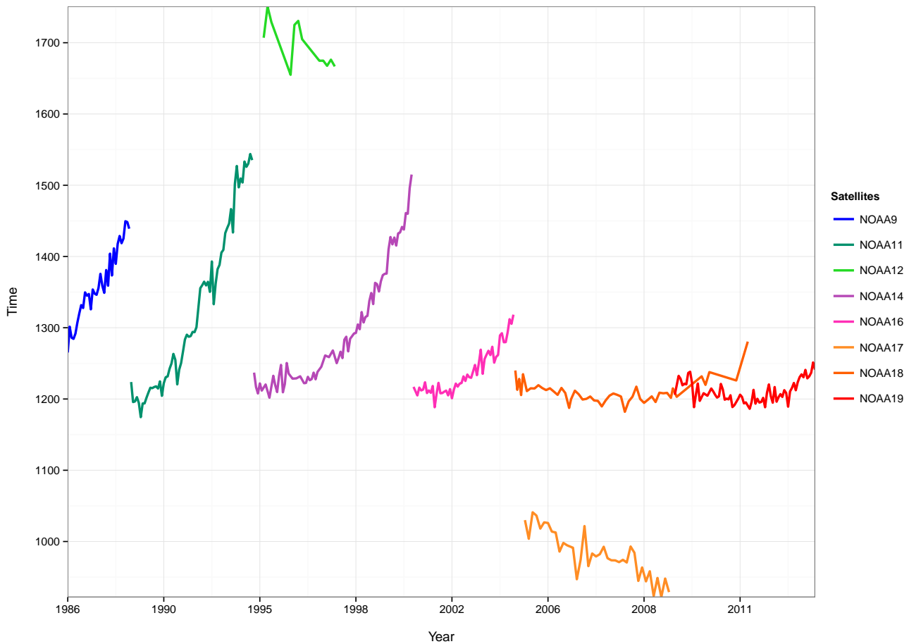
Figure 2.1: Plot of variation in observation times of National Oceanic and Atmospheric Administration (NOAA) instruments, note the large orbital drifts of the earlier NOAA-9/11/12/14 instruments.
