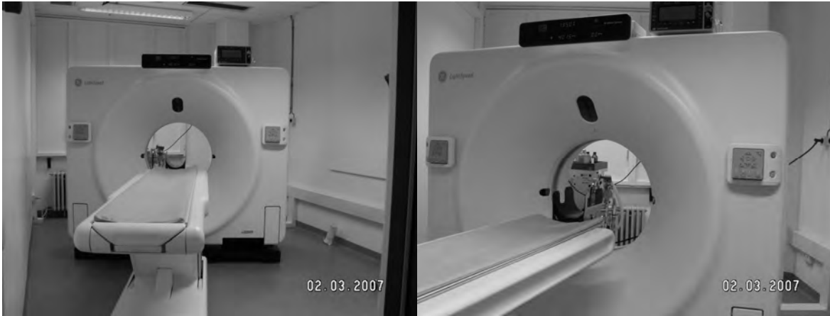
Fig. 18 The third-generation CT scanner (GE light speed) which was used in this experiment
