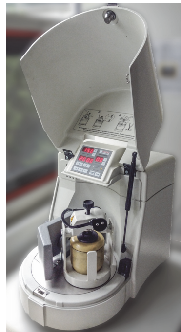
Figure 3.1 Picture of the planetary ball mill with opened lid containing the milling jar.
