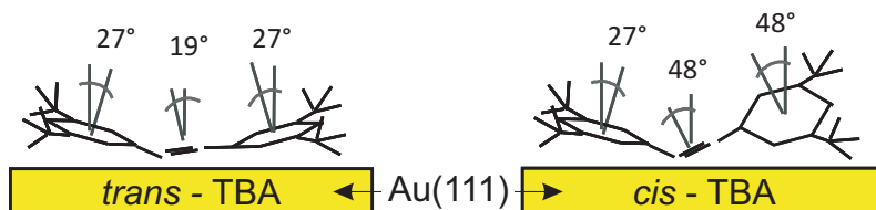
Figure 4.18: Absorption geometry of trans and cis-TBA in the monolayer phase. The given values represent the tilting of the phenyl ring normal and the azo-bridge normal in respect to the surface normal. Sketch courtesy of Roland Schmidt, MBI Berlin.
