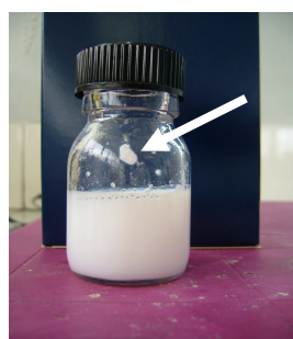
The picture of the flask shows polymer agglomerates, which are visible macroscopically.
