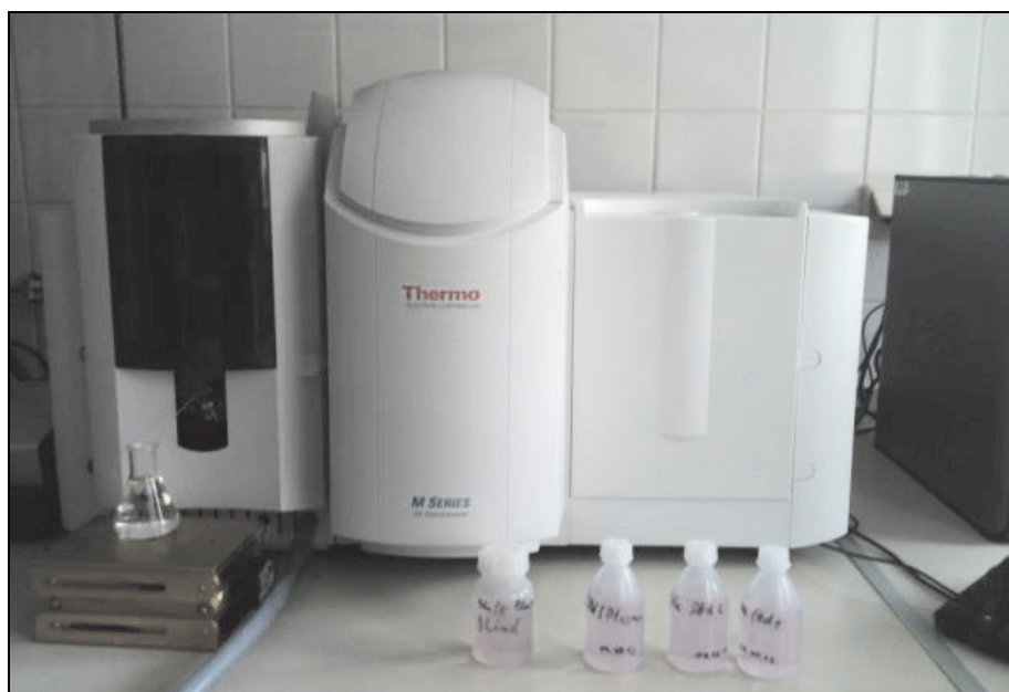
Figure 3. Flame atomic absorption / emission spectroscopy, (AAS, SOLAAR M6, Thermo Fisher Scientific, Cambridge, United Kingdom) used in emission mode for measuring total potassium and sodium concentrations in diluted bovine plasma samples
