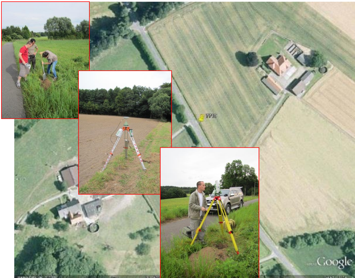
Figure 104: Surveying the reference points at field, required for geo-referencing the terrestrial dataset
