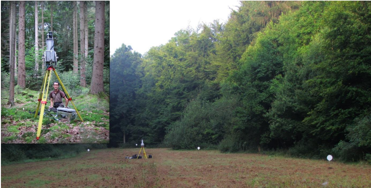
Figure 105: Terrestrial laser scanning of the targets in the clearing area for the global registration (right) and the single trees within the stand (left)
