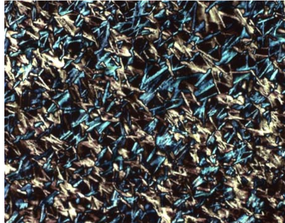
h. E7 on heating at 200 °C (magnification 50×)
