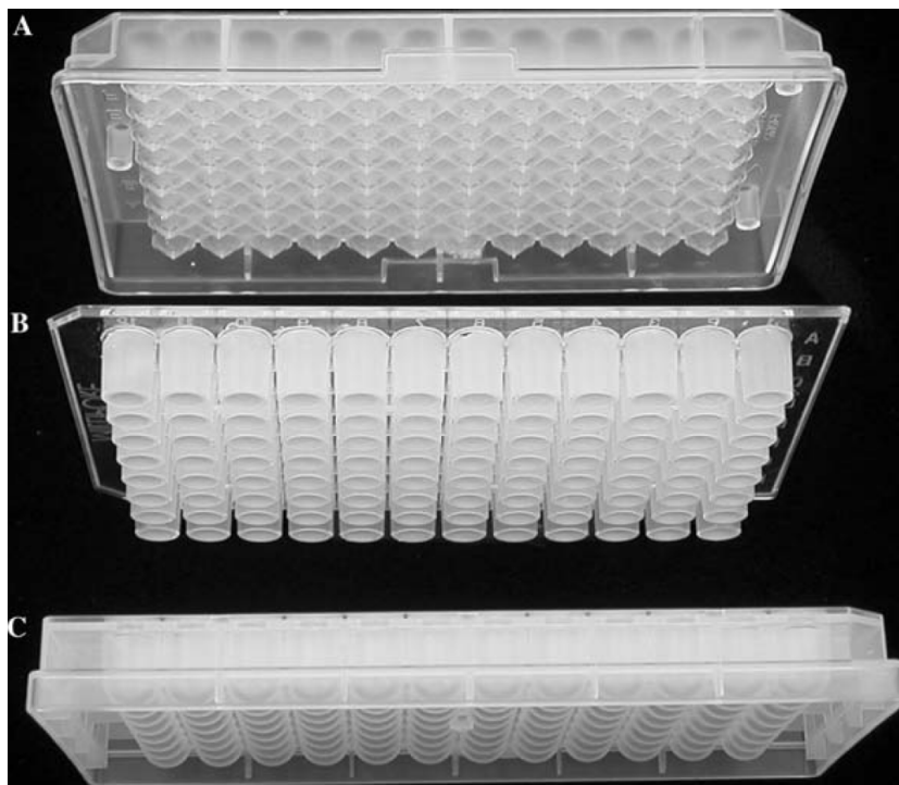
Figure 66: SpeedScreen “sandwich” assembly. Pinhole plate (A), size-exclusion chromatography plate (B) and collection plate (C), for processing all samples simultaneously in the 96-well format [156] .
