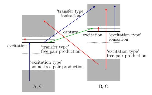
FIGURE 5.7. The two-centre approximation of the free-particle scattering channel C. Ionisation and pair creation processes may be of 'excitation'- or 'transfer'type. A similar schematic picture has previously appeared in [EIC95].
