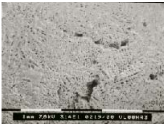
Figure 3.16 SEM pictures of sponges prepared with (A, B) 10% RG 503H in acetic acid at slow freezing rate; (C, D) 10% RG 503H in 1,4-dioxane and at slow freezing rate; (E) 10% RG 503H in 1,4-dioxane at fast freezing rate.
