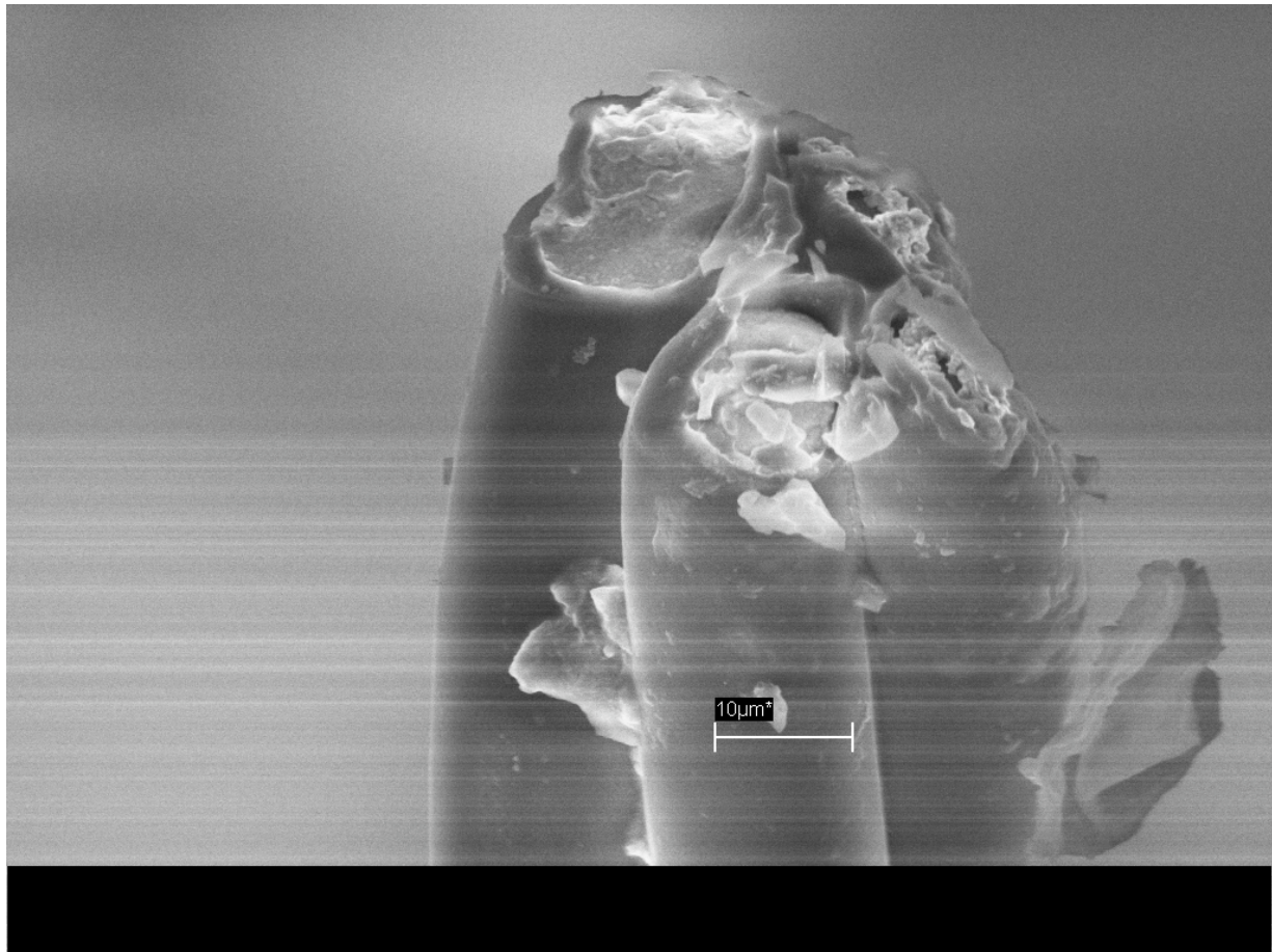
Fig.2: A scanning electron microscope picture from a partially plated tetrode. The polyurethane insulation was melted by heat to fix the coiled structure of the electrode bundle. Both electrodes on the right side show a wobble-like surface texture, due to the gold-PEG plating procedure (Ferguson et al., 2009). The scale bar indicates 10 \mu m. (Picture kindly provided by H. Hilger)
