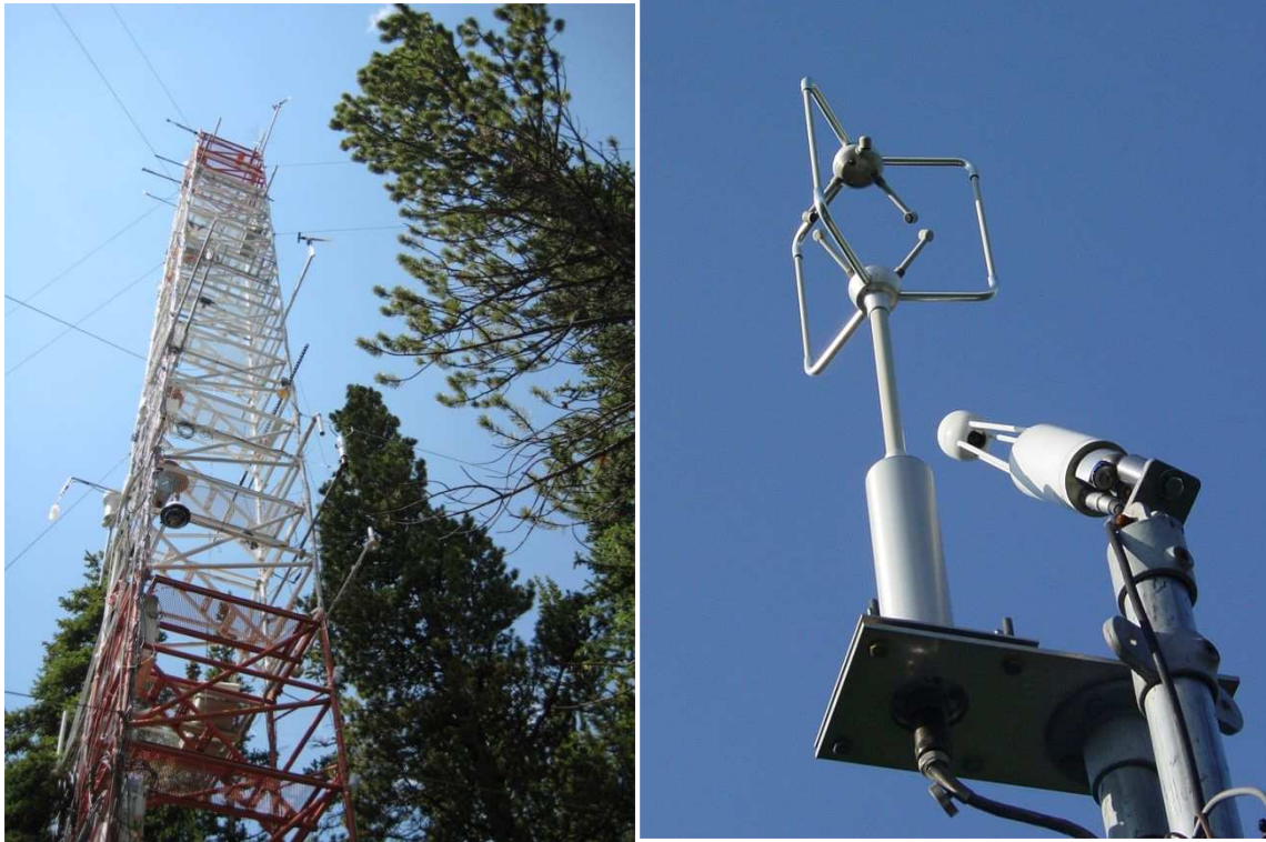
Figure 5. Niwot Ridge Ameriflux tower: located in Colorado, USA ( biocycle.atmos.colostate.edu ) and eddy covariance system: ultrasonic anemometer and infrared gas analyser ( en.wikipedia.org ).
