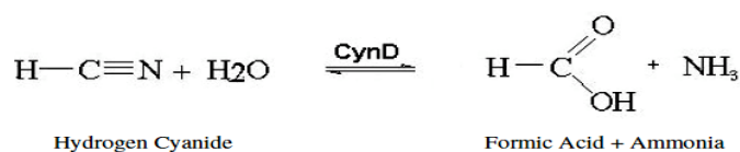
Figure 9.4b: Cyanide hydrolysis by cyanide dehydratase (CynD) to formic acid and ammonia.
