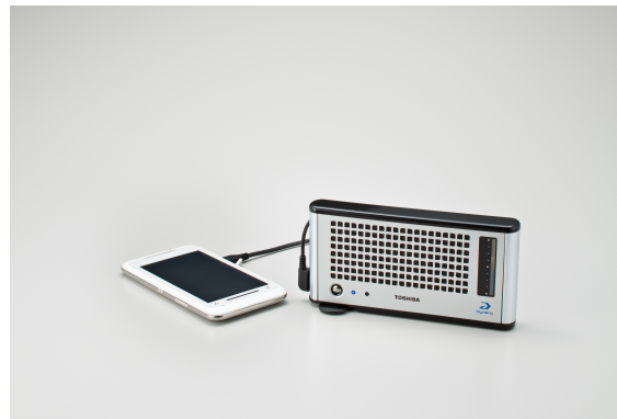
(d) Toshiba's DMFC powered cellphone charger [20]
