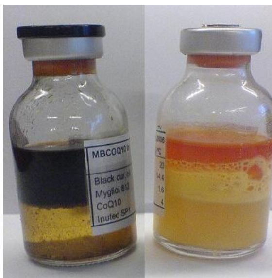
Figure 4-10: The reference emulsion samples after 1 year storage at 50°C. A change in the Q 10 color from orange to dark brown was observed in the sample stabilized using Inutec SP1 (the vial at the left). The sample stabilized using PlantaCare 2000 had a normal color (the vial at the right).
