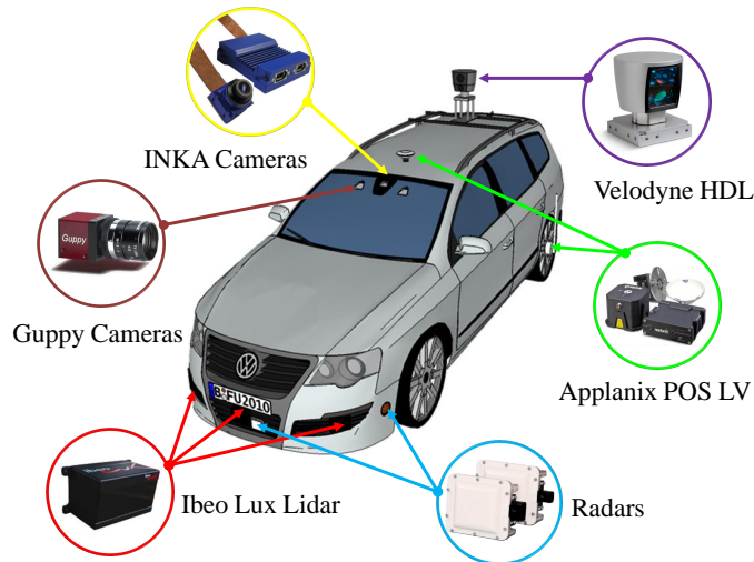
Figure 3.1: Sensor set-up of MadeInGermany 7 . Only the externally-visible part of sensors are illustrated.
