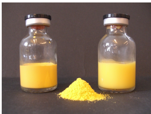
Fig. 4.51 Coenzyme Q10 nanosuspensions (formulation J) with a particle size of 219 nm (left), lyophilized CoQ10 nanocrystal powder (middle) and re-dispersed lyophilized CoQ10 nanocrystals (addition of 5% lactose) with a particle size of 263 nm (right).
