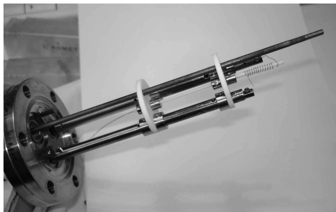
Figure 3.3: Picture of the inner parts of the gold evaporator that was used in the present thesis.
