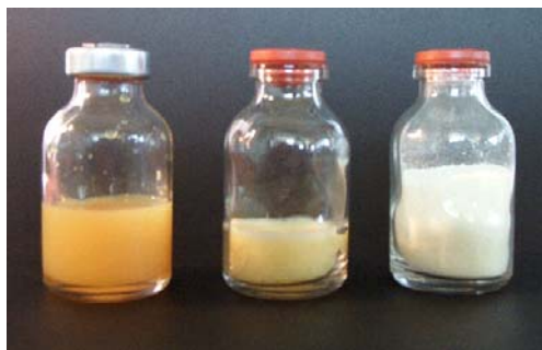
Figure 2-7: Amphotericin B nanosuspensions composed of liquid PEG 400 (left), as solid dispersion in solidified PEG 1000 (middle) and in form of ground solid PEG 1000 yielding a white powder (right) (with permission after (Bushrab 2003)).
