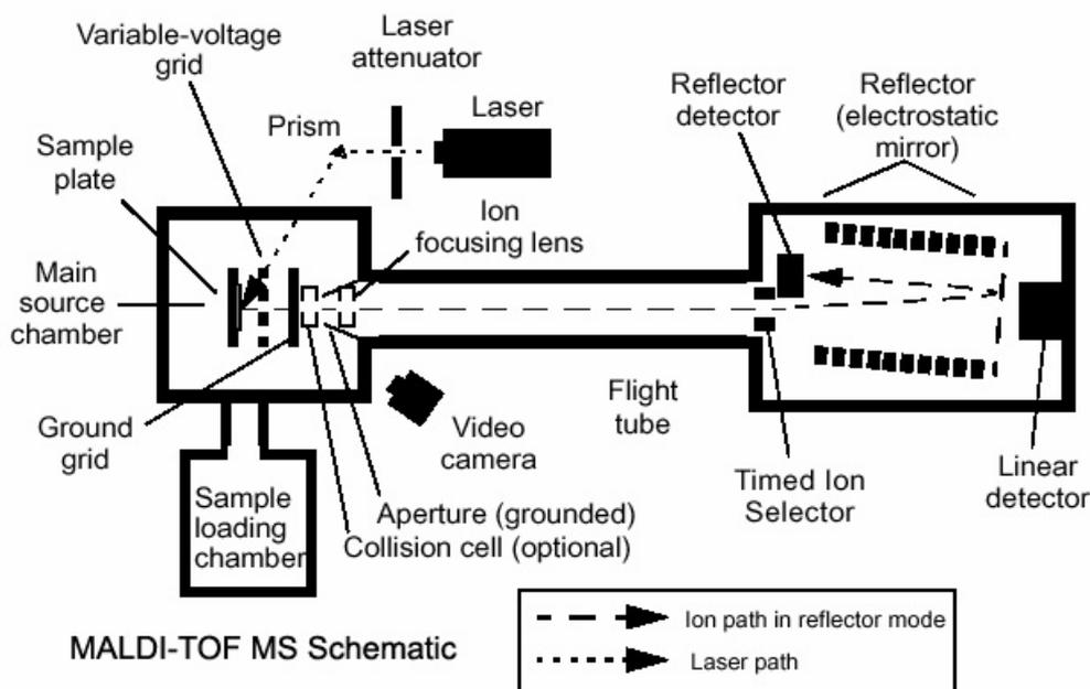
**Figure 4:** *Schematic illustration of MALDI-TOF-MS* The peptides applied to the sample plate (at the left) are desorbed and ionized by a laser pulse. After acceleration by a variable voltage grid they fly in high vacuum to the detector at the right. The times of flight of the analytes are translated to masses and acquired spectra are used for peptide mass fingerprinting.
