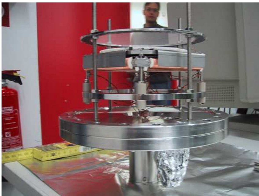
Figure 2.23: Photograph of the position sensitive detector and flange from the side. From top to bottom: mesh, MCP stack, delay-line anode, insulating ring, flange, and electrical feedthrough.
