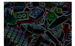
Figure 2.2.7: Shown are the borders found by a border detection algorithm applied to a picture of Lego bricks.
