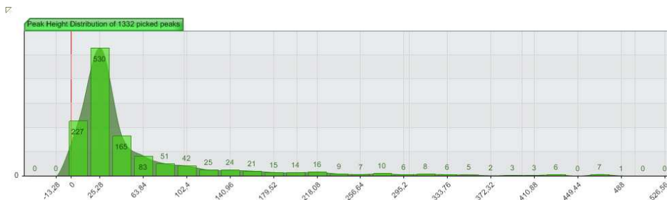
Figure 3.4.10: Histogram of peak heights from a randomly chosen spectrum. Note that only peaks smaller than 500 are displayed. The curve in darker green is a spline based approximation to the top mid-points of the histogram bars.
