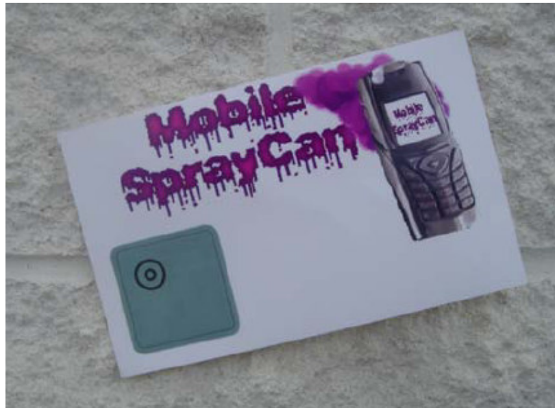
Figure 3.2. Exemplary picture of a passive RFID tag from [Garn 2006], the tag itself is located within the paper bag on the bottom left-hand side
