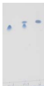
Figure 3.10: Separation of ETD from CON by using mobile phase (toluene: acetone, 1:1 v/v) and TLC plates.
