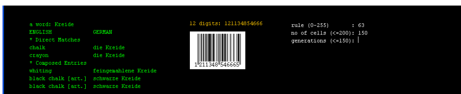
Figure 2.13: Left: CGI request (parameter prompt text “a word:”, user input “Kreide”) and answer from a CGI script using the Leo [52] server. Center: CGI request (prompt “12 digits:”) to a CGI returning a EAN code graphic and its result. Right: CGI request for a CGI with several parameters, with the third parameter not yet entered by the user.
