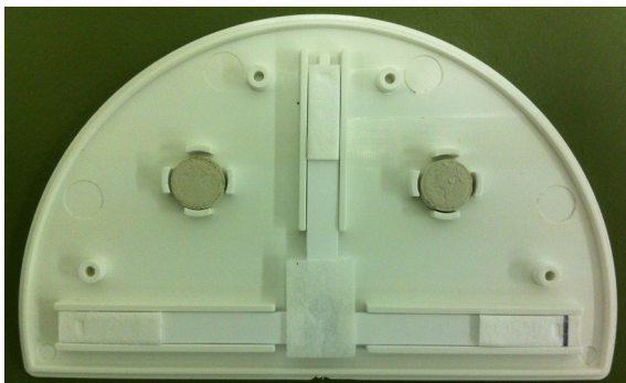
Figure 1 RapidVet-H immunochromatographic feline blood typing cartridge, opened
