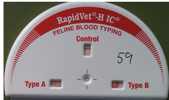
Figure 5 RapidVet-H immunochromatographic feline blood typing cartridge showing the test of an AB sample
