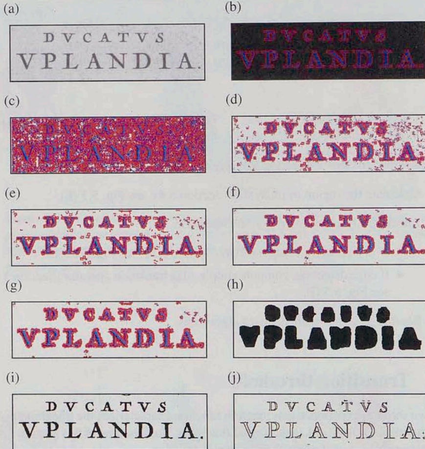
Figure 5.5 – (a) Original image. (b) Transition image by function maxmin with neighborhoods of radius 2. (c) Transition image. In blue, pixels with transition value higher than zero; in red, pixels with transition value lower than zero. (d) The transition image after filtering by t_+ = 14 and t_- = 15 . (e) Transition image after removing isolated pixels. (f) Transition image after incidence transition operators. (g) Transition image after dilation transition operators. (h) Region-of-interest image. (i) Binary image by modeling the gray intensities as lognormally distributed. (j) Edge image.
