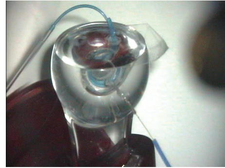
FIGURE 1: Cochlear model with positioned sensor and an inserted probe electrode.
