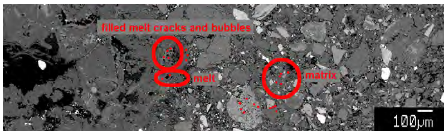
Fig. E.8.: FBN73: Points of EMPA measurements of melt particles and suevite matrix drawn in BSE images. 380-602 m depth.
