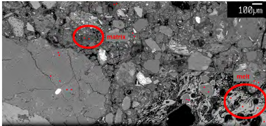
Fig. E.20.: Otting: Points of EMPA measurements of melt particles and suevite matrix drawn in BSE images. 1.8 m depth.
