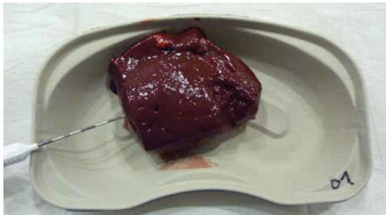
Figure 2. Example of an ex vivo bovine liver specimen in a kidney basin with a microwave ablation antenna positioned in the center before microwave ablation.
