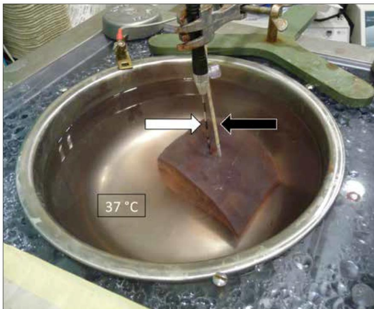
Figure 4. RFA setup: metal bowl filled with 0.9% saline, heated to 37°C to simulate physiological body temperature, current flow and heat conduction, cuboid liver specimen, and RF electrode (white arrow). To further validate the temperature inside the parenchyma, a fiberoptic measuring system (Neoptix, Québec, Canada; black arrow) was positioned inside the parenchyma 1 cm from the expected center of each lesion.
