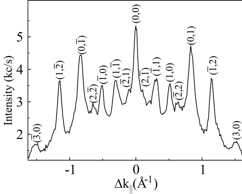
**Figure 4.10:** He diffraction spectrum from the 2-fold  $d$ -Al<sub>71.8</sub>Ni<sub>14.8</sub>Co<sub>13.4</sub>(001 $\bar{1}$ 0) surface along the quasicrystalline [10000]-direction at 21 meV He atom kinetic energy. The peaks are at  $\Delta k_{\parallel} = 0.51(m + n\tau) \text{ \AA}^{-1}$ , with  $m$  and  $n$  integers. Values of  $m$  and  $n$  are shown above the peaks.
