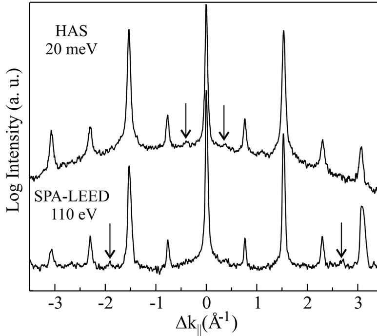
**Figure 4.9:** A comparison between HAS and SPA-LEED along the periodic [00001] direction (upper: He diffraction at 20 meV beam energy and lower: Electron diffraction at 110 eV electron energy). Weak peaks indicated by arrows correspond to a 16 Å periodicity.
