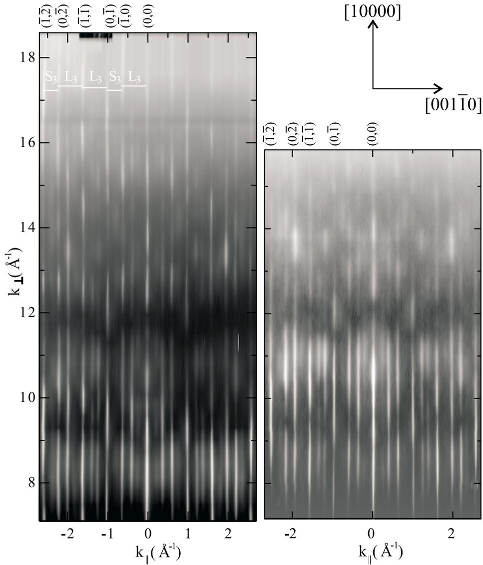
**Figure 4.5:** A gray scale plot of LEED intensity  $I(k_{\parallel}, k_{\perp})$  with  $k_{\perp}$  along  $[10000]$  (vertical) and  $k_{\parallel}$  along  $[001\bar{1}0]$  (horizontal). Left:  $0^{th}$  order spots (spots on the  $0^{th}$  column of SPA-LEED image, Figure 4.2) and right:  $2^{nd}$  order spots (spots on the  $2^{nd}$  column).
