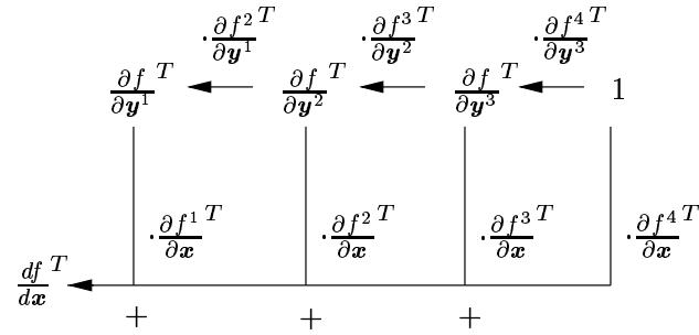
Figure B.3: Computational graph of the reverse mode of differentiation.
