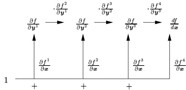
Figure B.2: Computational graph of the forward mode of differentiation.
