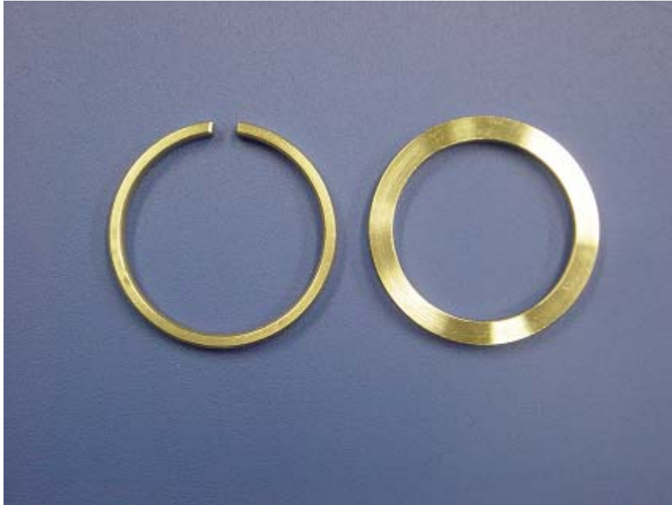
Figure 4 Two metal rings used in cell seeding. The left ring with a 7mm wide gap was positioned under the patch with outer diameter of 44 mm and inner diameter of 40 mm. The second ring was placed upon the patch with outer diameter of 44 mm and inner diameter of 34 mm. The height of both rings was 5 mm.
