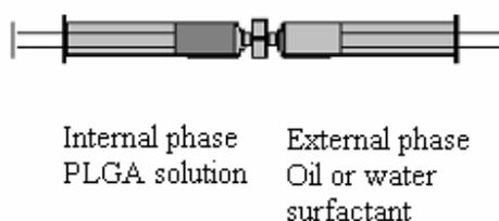
Fig. 9. Two syringe system for preparation of in situ forming microparticles.
