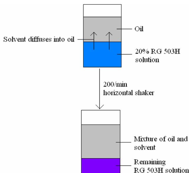
Fig. 10. Experiment set-up to determine the diffusion rate of solvent from polymer solution into different oily external phases.
