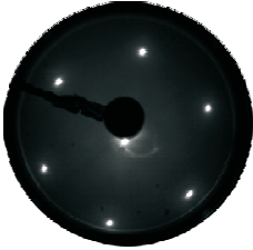
Figure 21: LEED image at 91.1 eV electron energy of a graphene layer on Ni/W(110).
