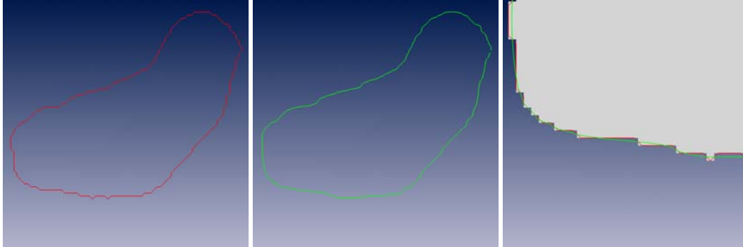
Figure 4.8: A binary border initialization as used in standard distance map algorithms is not suitable for extrapolation, because it implicitly defines a jerky contour (left). After smoothing the contour is still compatible with the labeling (right) but significantly smoother (center).
