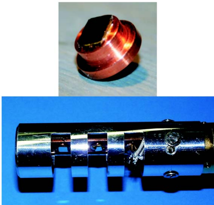
Figure 5.6: Photograph of the used sample holder. Top: Copper disc with glued EuTe sample. Bottom: Copper block connected to the cryostat with two mounted EuTe samples (left and center slit) and the silicon diode temperature sensor (right slit). The whole sample holder is shielded by an aluminum tube with only three horizontal slits to perform the scattering experiment.
