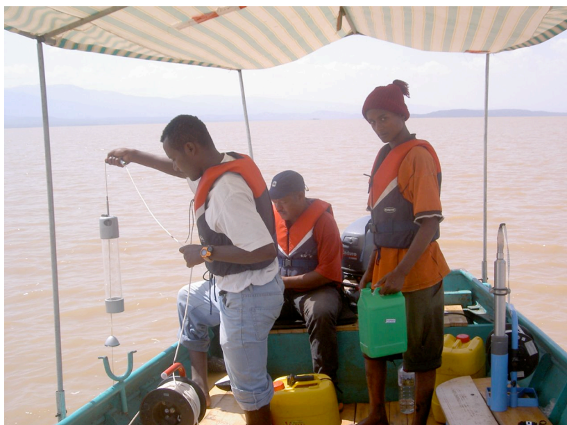
Figure 4.5. Water sampling from fixed monitoring station.
