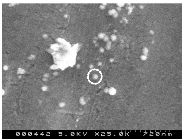
Figure 4.3. SEM image of a Bi deposited Pt surface.
